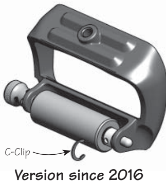
Figure 2: Removing the C-clip.
